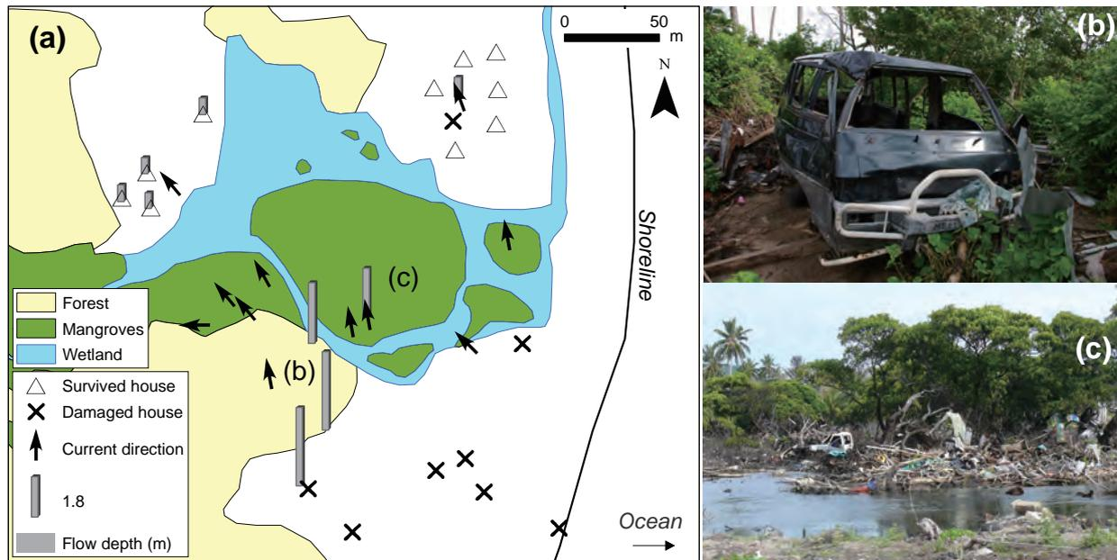
**Fig. 4** Tsunami damage around mangrove forest in Lotopu'e. (a) Tsunami flow depth, current direction (the arrows do not include a flow strength) and house damage. (b) and (c) show a car and many pieces of debris drifted into the mangrove forest.
