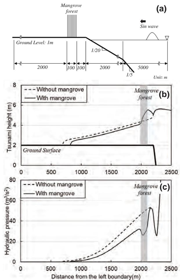
**Fig. 5** (a) Numerical conditions of the cross-sectional simulation. (b) Numerical results of the maximum tsunami height and (c) hydraulic pressure with/without mangrove forest. Solid and dotted lines show numerical results with and without mangrove forest, respectively. The shaded area indicates the location of the mangrove forest.
